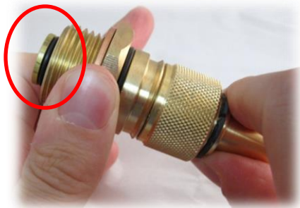
Plug with Sampler attached showing the valve being opened
